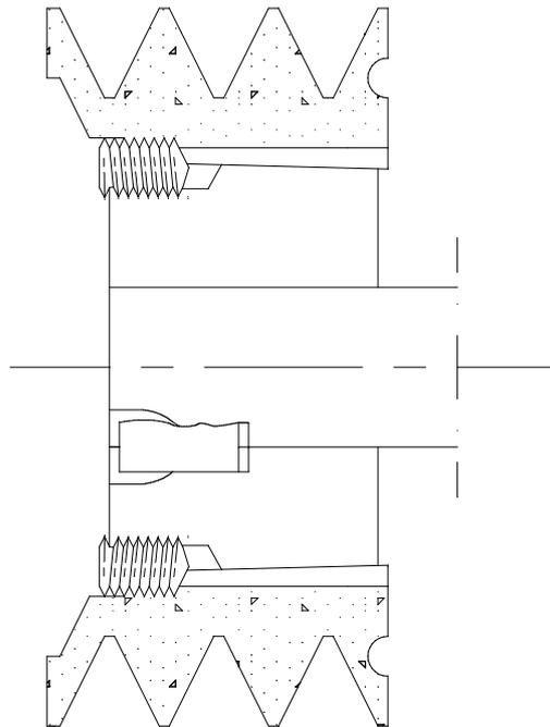
**Design:** Consists of a slotted cast-iron sleeve with a keyway in the bore and two half threads and two screws on the OD. The OD is tapered. The bore in the hub has the same half threads and taper.
