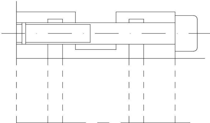
This type differs in design to most other mechanical types as it just consists of one piece of steel. When tightening the screws the whole sleeve is pressed together and also into contact with hub and bore. It is mostly sold to the machine tool industry where the compact design gives some design advantages.
