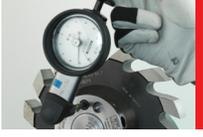
Let the tool set cool down and lock the screws with Loctite or equivalent and tighten them to min 8 Nm (70 lbf.in).
