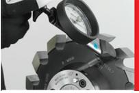
**4.** Mount the whole unit onto the grinding machine spindle. Tighten the pressurizing screw until it stops, max 10 Nm (7.4 lbs). Any higher tightening force will not increase the fastening force.
