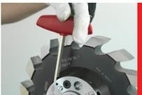
**6.** Release the pressurizing screw with an Allen T-wrench. Remove the tool unit from the grinding machine and it is now ready to be installed on the machine.
